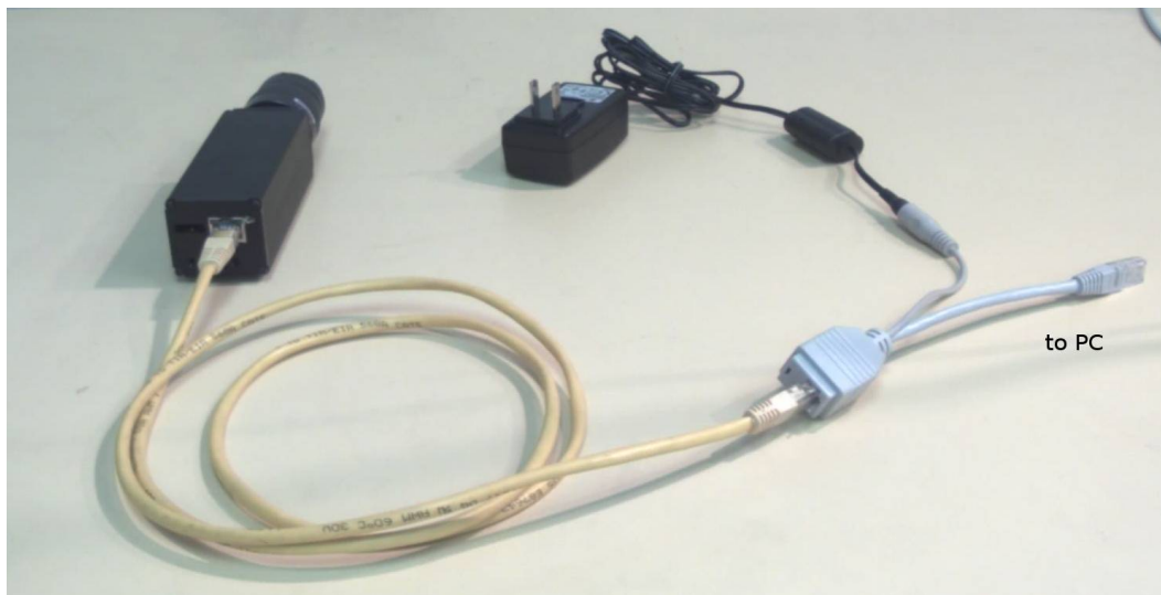
Fig.3 Camera connection using a PoE Switch
