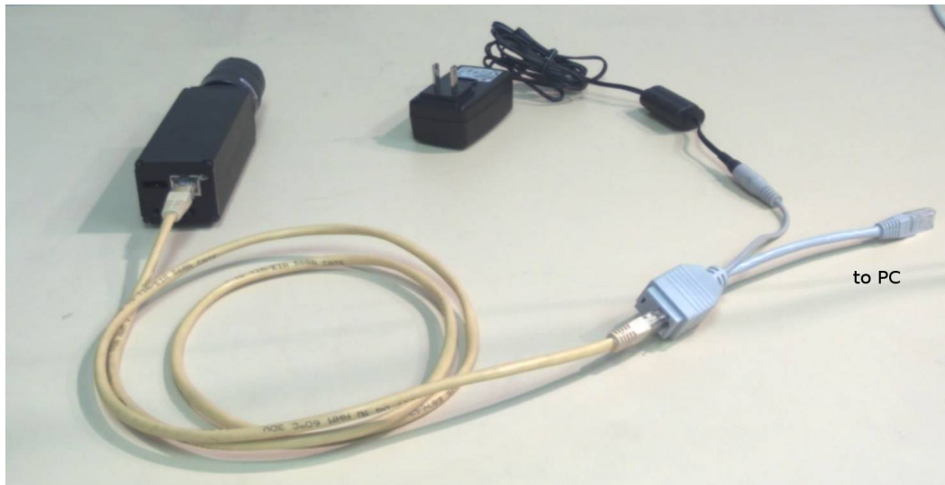
Fig.3 Camera connection using a PoE Switch
