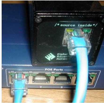
Fig.2 Camera connection using a PoE Switch (just plug the camera directly to the switch)
