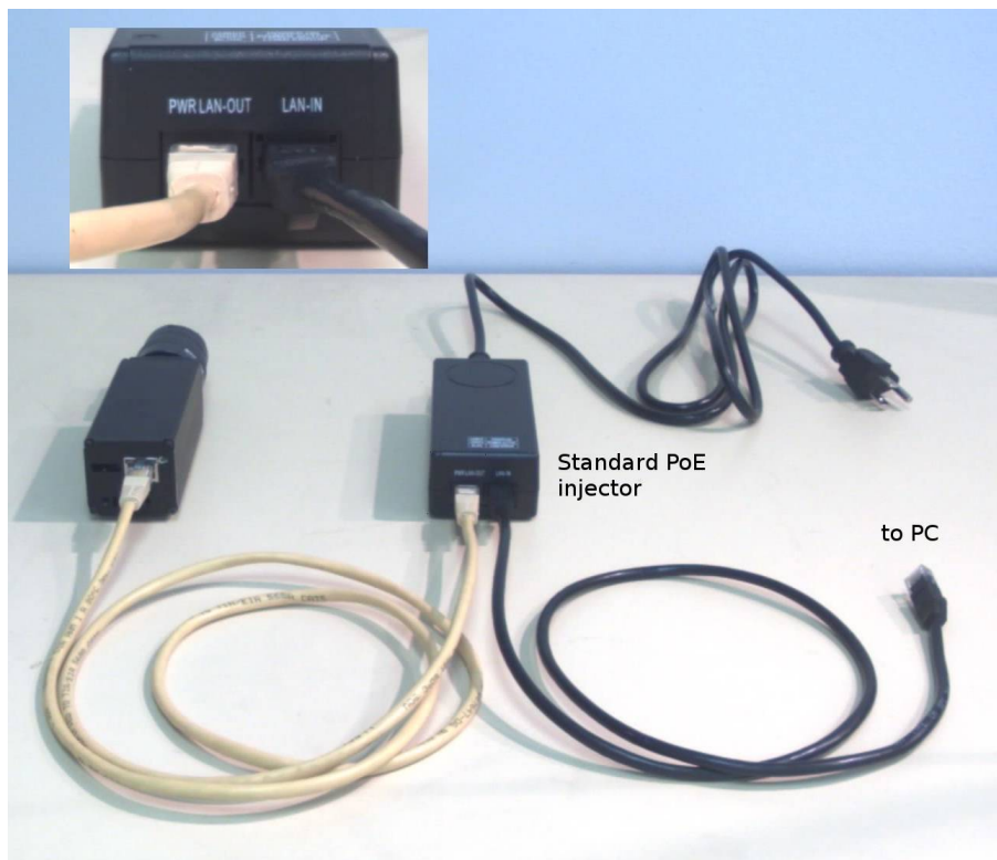
Fig.1 Camera connection using a standard PoE Injector
